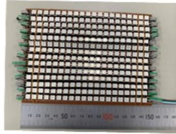
Fig. 5. LED matrix array
