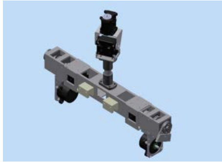
Fig.4. The shoulder and neck mechanism
