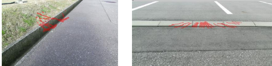
Fig.9. The results of detection of 25 [mm] difference in level by the Rolling 3D Lidar
